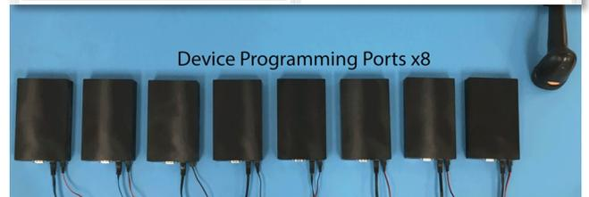
*Encrypt and program multiple devices in parallel*
