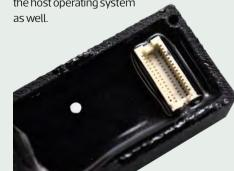
The high-density connector is surprisingly robust for its small size
